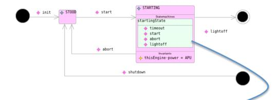
The starting process is elaborated by adding a statemachine startingState inside STARTING. This addition is quite simple because it doesn't depend on any other feature such as the power source so we decided that a separate refinement wasn't necessary.
